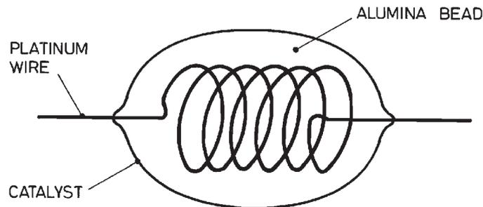
The design has been modified to reduce the amount of power used by the sensor and to make the sensor more resistant to poisoning and mechanical shock. SGX, when known as E2V, was in the forefront of these developments and the current range of pellistors incorporates the design improvements.
