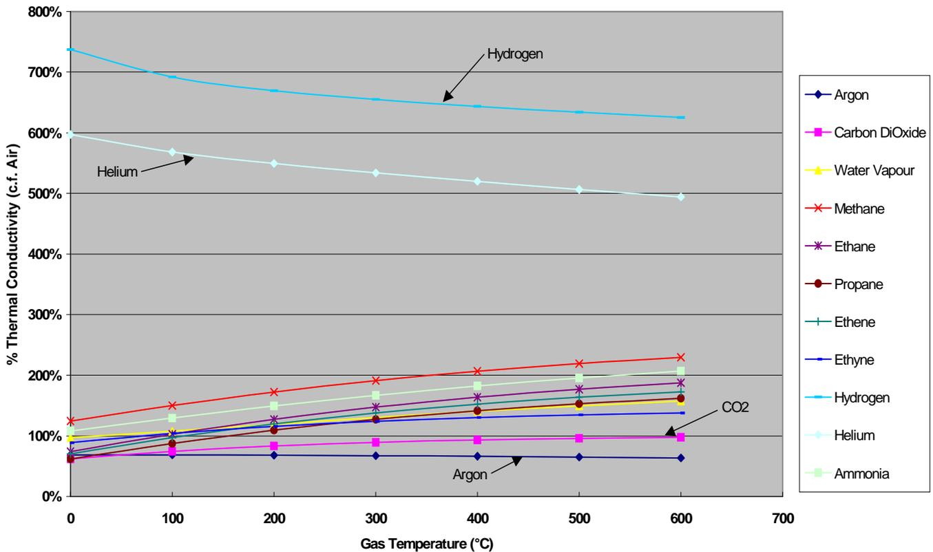
As shown above, gases with a low density (and high thermal conductivity) such as hydrogen and helium will have much bigger sensor signals compared with other gases. The difference could be up to a factor of 6.
