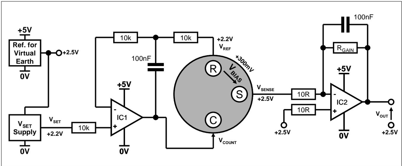
Figure 4 –Biased Sensor Circuit with Single Power Rail
