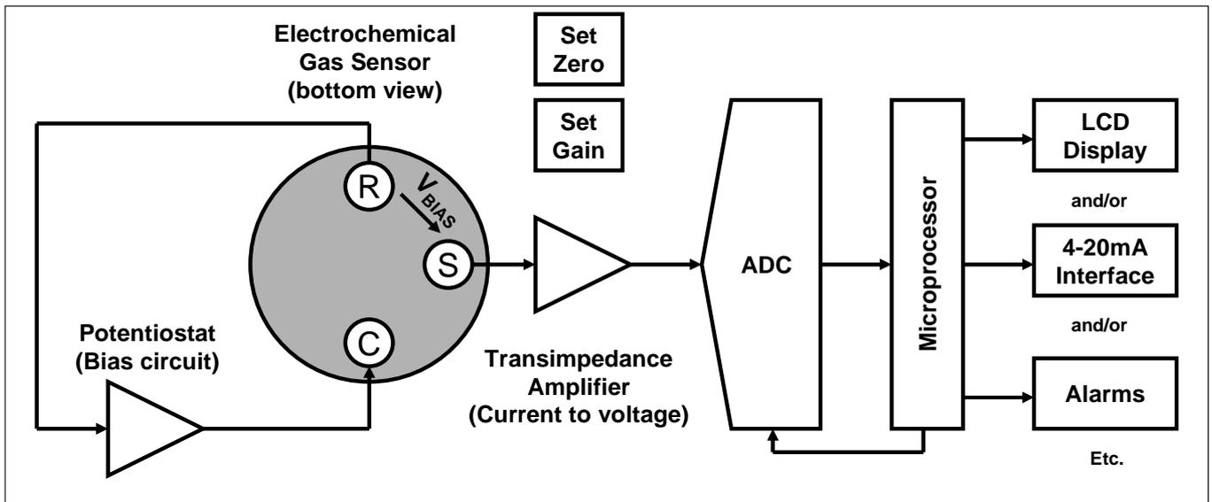
Figure 1 – Block Diagram of Typical Gas Detection System using an Electrochemical Gas Sensor
