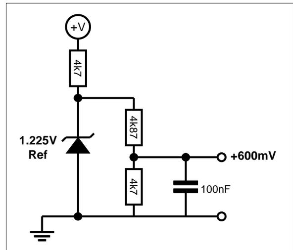
Figure 6 – Example Bias Circuit for  $+600\text{mV}$
