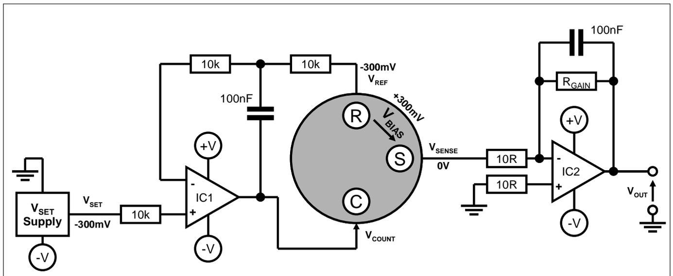
Figure 3 – Biased Sensor Circuit with Split Power Rails
