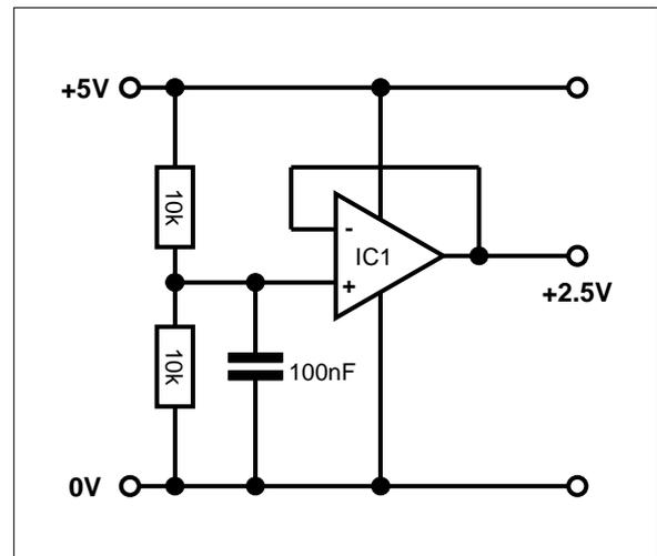
Figure 7 – Example Circuit to Generate Virtual Ground
