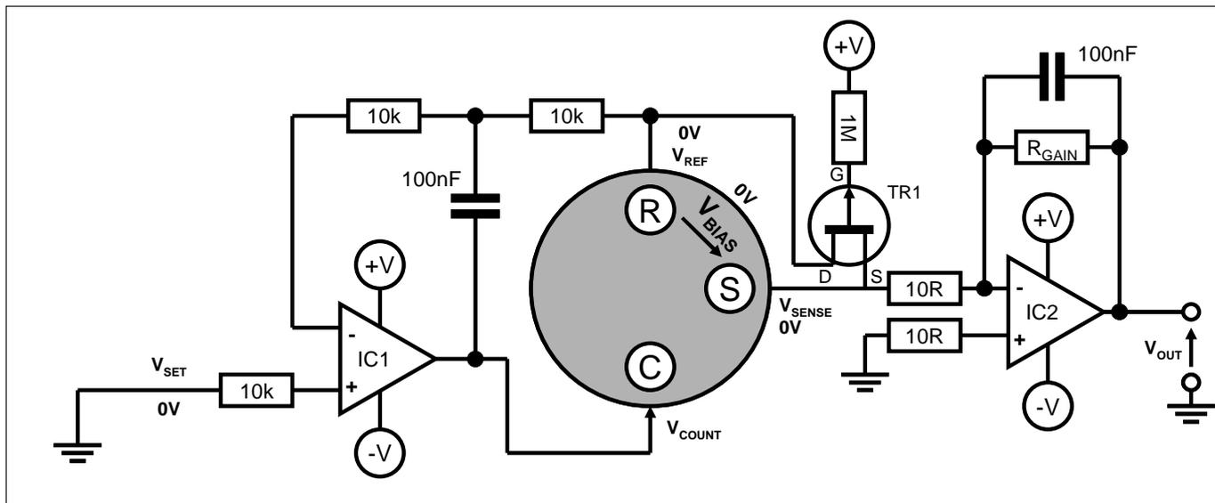
Figure 2 – Unbiased Sensor Circuit with Split Power Rails
