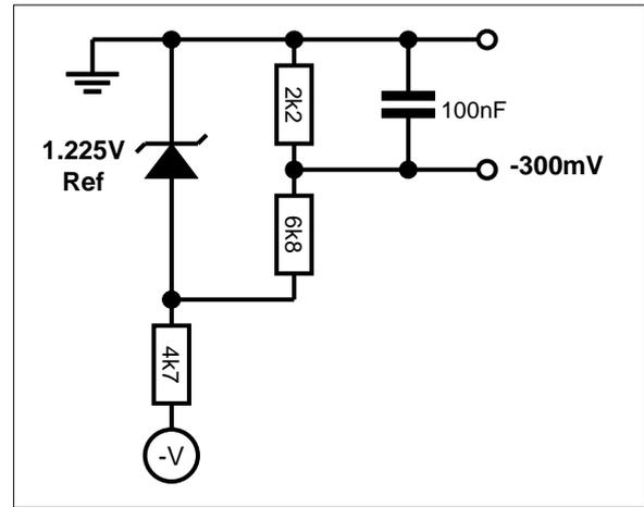
Figure 5 – Example Bias Circuit for  $-300\text{mV}$
